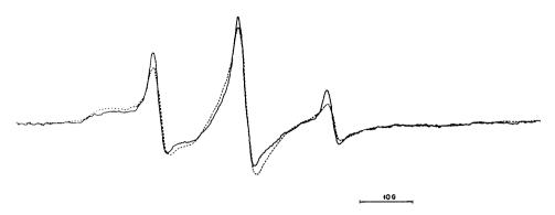
Fig. 1. Spectra of MSL-6 in plasma membrane from smooth muscle of guinea pig ileum suspended in Tyrode solution. Solid line – in the absence of AII; dotted line – in the presence of a 1 mM solution of AII. Experimental conditions are given in the text.
